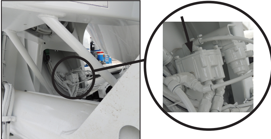
Figure 1: R-12 Valve inside the rear pedestal has a flat top.
