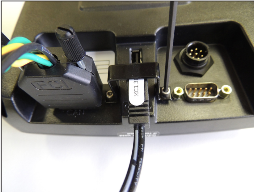
Figure 2: Install the bracket and screws. Do not over tighten screws.
