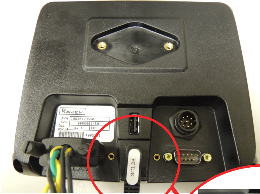
Figure 1: Locate the predrilled holes around the power plug on the back of the monitor.
