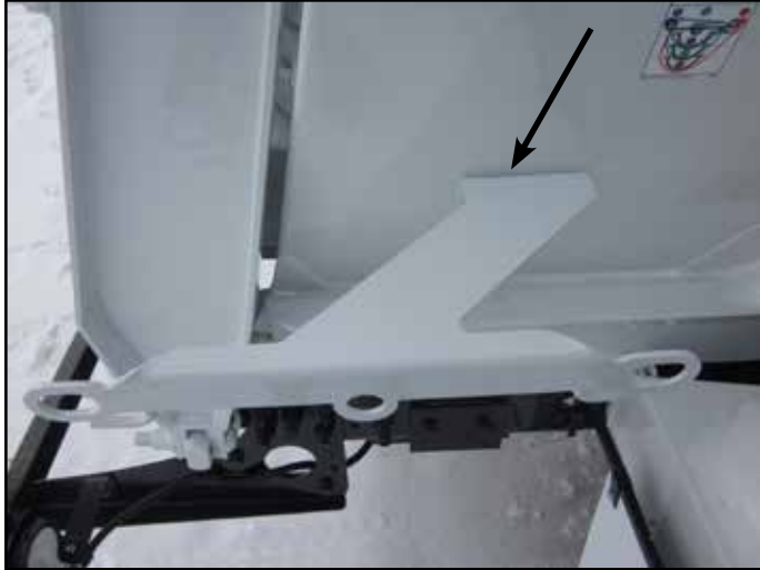
Figure 4: Offset Style Chute Stop must be replaced.
