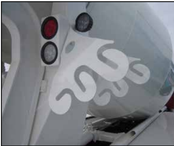
Figure 1: “Old” Style Chute Rack does not need to be replaced . On left is the three chute rack design, and on the right is the two chute rack design.
