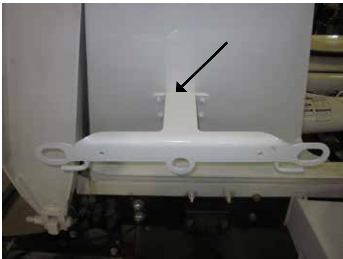
Figure 5: Straight Style Chute Stop does not need to be replaced.
