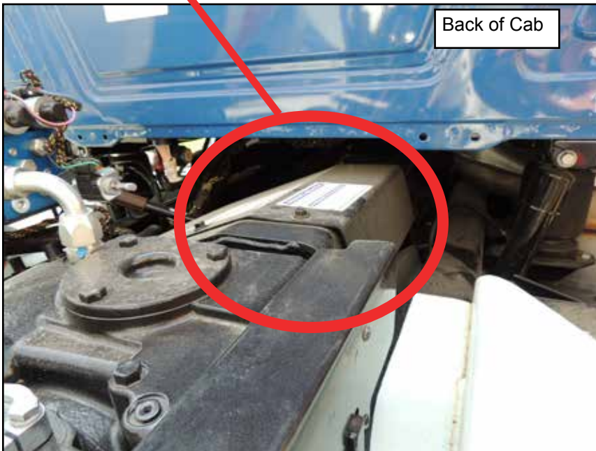
Figure 3: PTO drive shaft location (cover is on the shaft).
