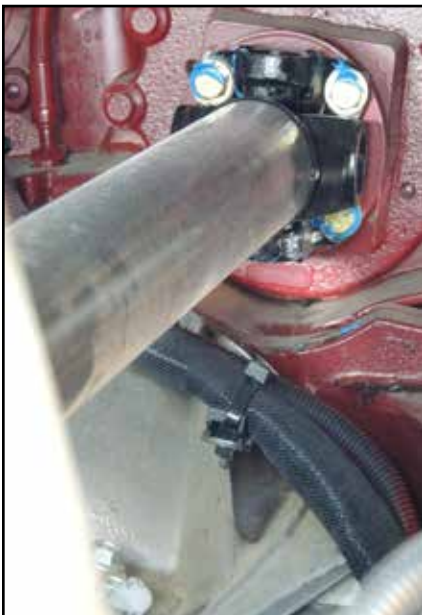
Figure 12: Representation: Use the PTO strap kit that attaches the drive shaft to the pump.
