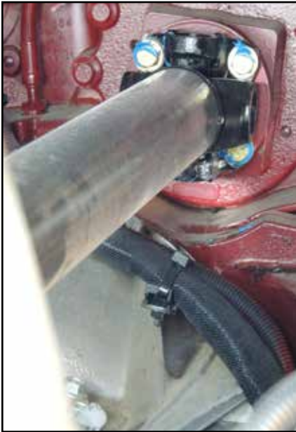
Figure 9: Representation of the four bolts and washers that attach the drive shaft to the pump.
