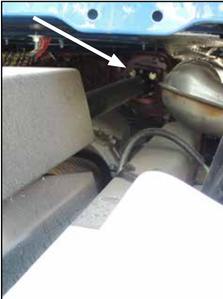
Figure 11: Four bolts and washers that attach the drive shaft to the REPTO (engine side).
