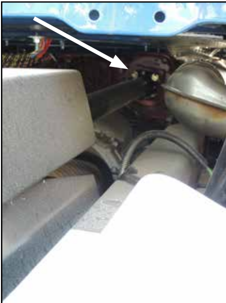
Figure 10: Four bolts and washers that attach the drive shaft to the pump.
