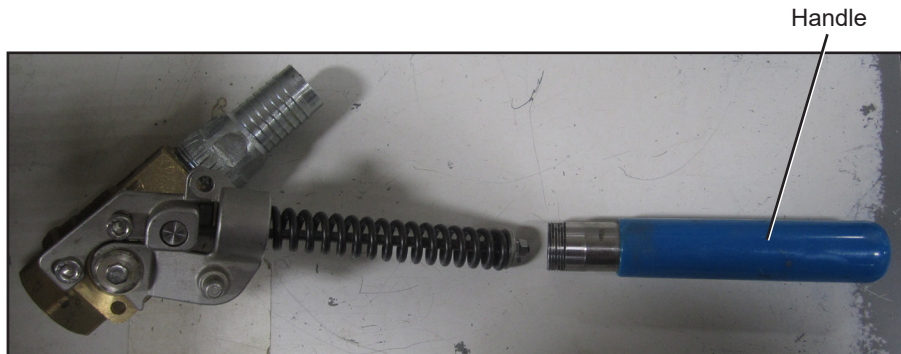
Figure 2: Handle Removed from Ball Valve Assembly..
